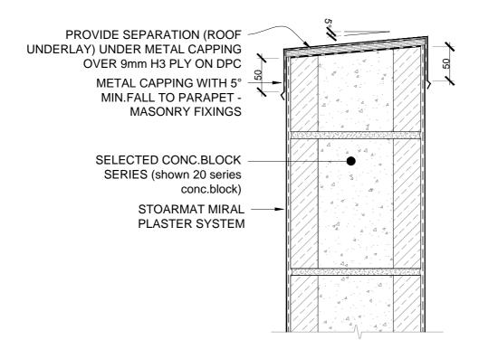
**NOTE**: CUT BLOCK TO SUIT OR BASECOAT PLASTER TO A FALL APPROX.18mm FROM FRONT EDGE BEFORE INSTALLING PLYWOOD ON DPC. ALTERNATIVELY USE H3.1 TIMBER PLATE, MAINTAINING FLASHING COVER OVER CONC.BLOCK OF 50mm MIN.
