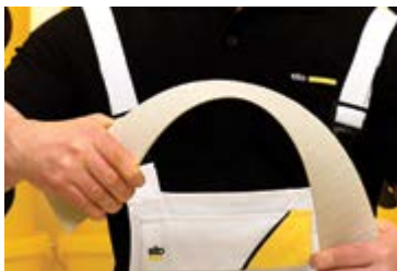
A bend test demonstrating the extraordinary elasticity and resultant high crack resistance of Sto synthetic renders.
