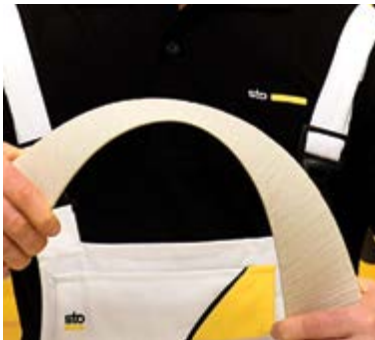
A bend test demonstrating extraordinary flexibility and an impact test proving high fracture resistance of StoArmat renders.
