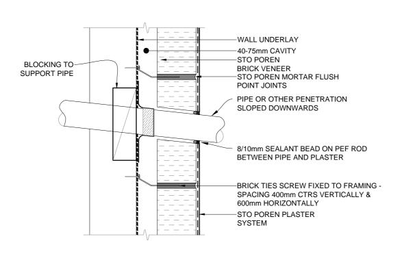
NOTE: INSTALL FLASHING TAPE WITH 100mm CLEARANCE AROUND PIPE ONTO WALL UNDERLAY AND WRAP 25mm ROUND PIPE.
