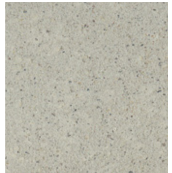
Stolit MP Natural: Coloured fine finishing render with a dark grain.
